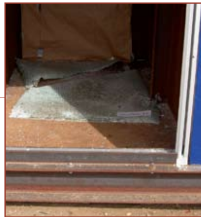
The effectiveness of security window film is shown in this sequence of photos taken during a test explosion. The window glass, attached to the security film, shatters but stays largely within the frame, as opposed to flying through the building's interior.
