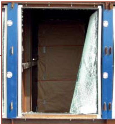
The effectiveness of security window film is shown in this sequence of photos taken during a test explosion. The window glass, attached to the security film, shatters but stays largely within the frame, as opposed to flying through the building's interior.
