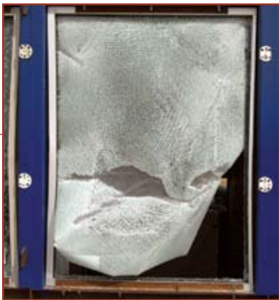
The effectiveness of security window film is shown in this sequence of photos taken during a test explosion. The window glass, attached to the security film, shatters but stays largely within the frame, as opposed to flying through the building's interior.
